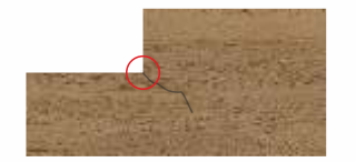
Crack arising due to L shape 90° cutting.
