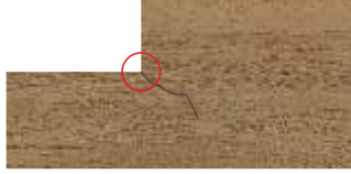
Crack arising due to L shape 90° cutting.
