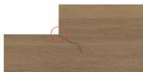
Crack arising due to L shape 90° cutting.
