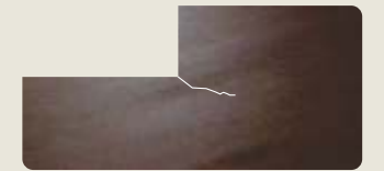
Cutting a laminate sheet at an angle of 90 degree leads to development of cracks in corner after pasting. Therefore it is advisable to avoid cutting at an angle of 90 degrees.
